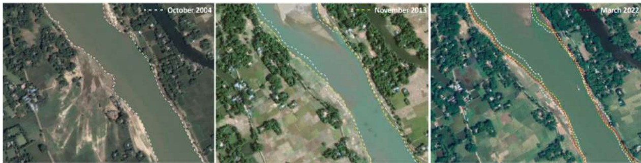
Figure 13: Riverbank erosion in Gaokandia Union (data from Google Earth Pro, 25°09'27.33" N 90°39'46.94" E)
